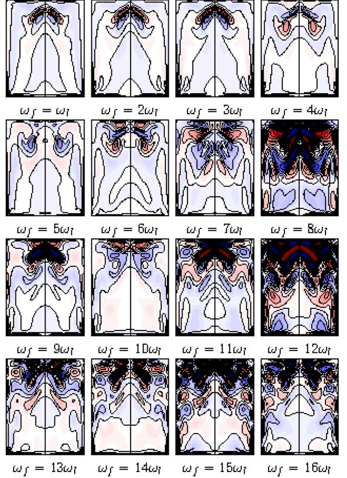
FIG. 4. (Color online) Vorticity field under linear parameter ramping. For  $P = 1$  [ $\omega_f(t) = \omega_0 + \epsilon t$ ], snapshots of the azimuthal vorticity field for various values of  $\omega_f$ , where  $\omega_l = \omega_b/2$ . Relatively strong vorticity fields are observed for  $\omega_f(t) = 8\omega_b$ ,  $12\omega_b$ , or  $15\omega_b$ , as in the corresponding stationary system (cf. Fig. 1).
