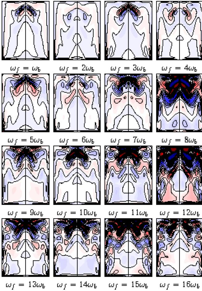
FIG. 1. (Color online) Structure of the azimuthal vorticity field in the stationary flow system. For  $Re = 2600$ ,  $H/R = 2.5$ , and  $A = 0.01$ , snapshots of the azimuthal vorticity modulation for various values of  $\omega_f$ :  $\omega_f = n\omega_b$  ( $n = 1, \dots, 16$ ), where  $\omega_b = 0.014\,544\,027\,777$ . For  $\omega_f = 8\omega_b, 12\omega_b$ , or  $15\omega_b$ , the vorticity fields are relatively stronger.
