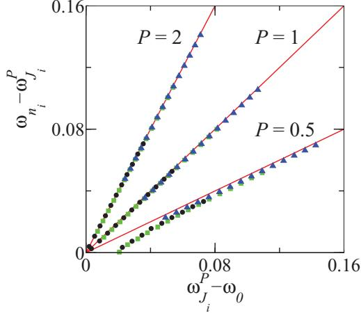
FIG. 7. (Color online) Verification of Eq. (12). Numerically obtained relation between  $(\omega_{n_i} - \omega_{J_i}^P)$  and  $(\omega_{J_i}^P - \omega_0)$  for  $P = 1/2, 1$ , and  $2$  and fixed  $\epsilon = 10^{-6}$ .
