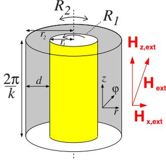
FIG. 1. (Color online) Schematic sketch of the Taylor-Couette system in a homogeneous magnetic field  $\mathbf{H}_{\text{ext}}$ .
